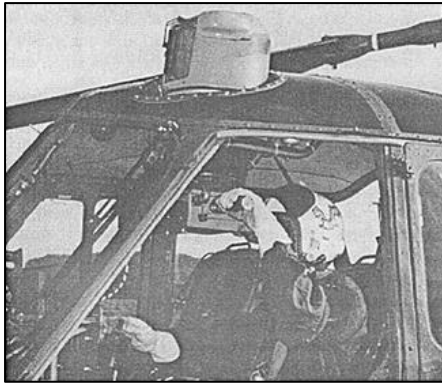
Air Gunner operating the Avimo/Ferranti AF120 stabilised sight.
